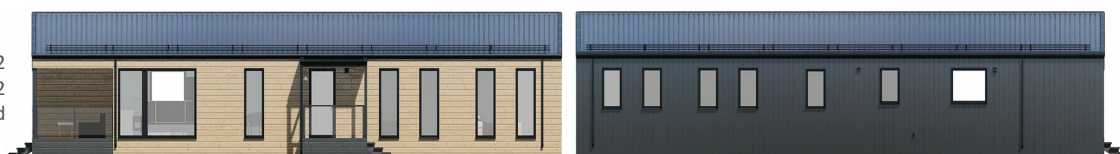
Type-6: metal profile roof, 1/2 metal profile facade + 1/2 horizontal wood
