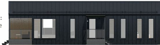
Type-2: clickfalz roof, clickfalz facade
