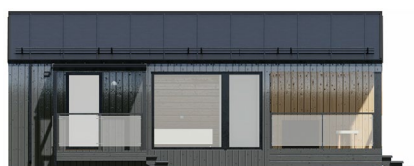
Type-10: clickfalz roof, 1/2 clickfalz facade + 1/2 vertical wood
