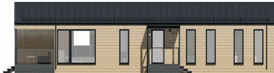
Type-3: palatinate roof, horizontal wood facade
