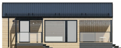
Type-6: metal profile roof, 1/2 metal profile facade + 1/2 horizontal wood
