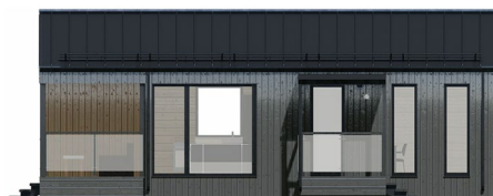
Type-4: palatinate roof, vertical wood facade
