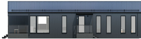
Type-1: roof metal profile, facade metal profile
