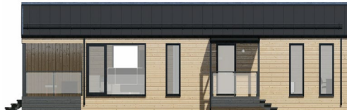
Type-3: palatinate roof, horizontal wood facade
