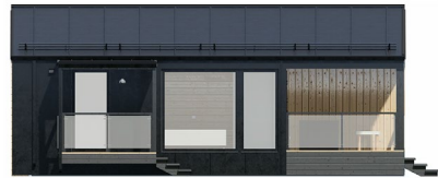
Type-2: clickfalz roof, clickfalz facade
